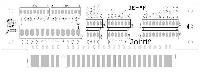
Compatible with 2.54mm (.100") pitch headers. A 3.96mm (.156") header can also be used for power. A 5mm LED can be used to indicate power on.
