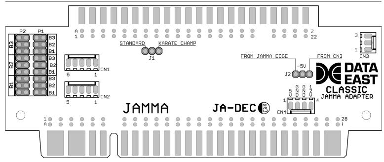
Designed to redirect DATA EAST Classic game PCB signals to work properly in a JAMMA cabinet or with a Supergun. This adapter features a button remapper, support for secondary joysticks and compatibility with a negatron circuit.
